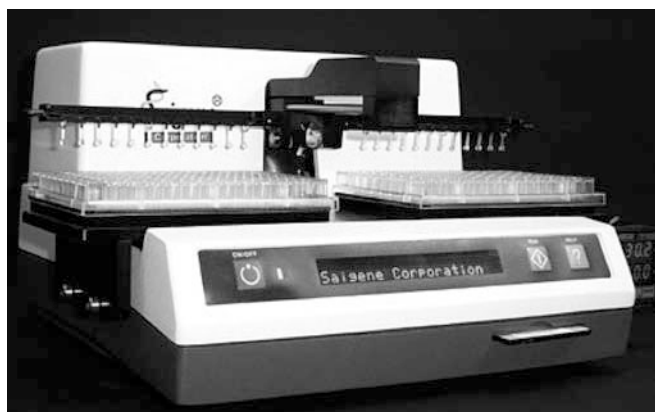
Fig. 11 Universal processor manufactured by Saigene for the automated performance of sandwich hybridization assays to detect HAB species. Samples are loaded into the first row of wells and a prong strip attached to each of the processor arms carries the probes and rRNA target through the assay reagents to yield a colorimetric signal for positive samples in the last row of wells. Photo courtesy of R. Gordon, Saigene
