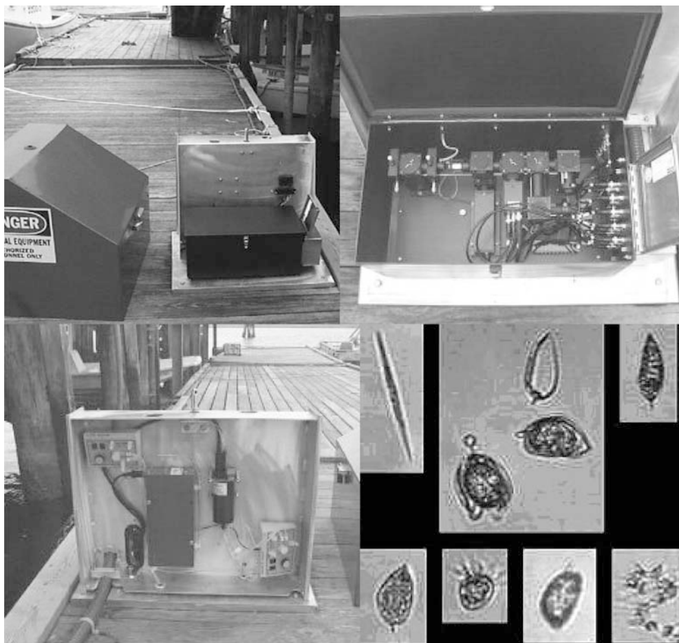
Fig. 9 Docktop flow cytometer and microscope (FLOWCAM) system developed by Fluid Imaging Technologies (FIT) ( top left ). Flow cytometer component ( top right ) and optical sensor component ( bottom left ) are contained in a weatherproof housing that can be equipped with wireless internet access. Sampling of up to 10 \text{ ml min}^{-1} can be pre-programmed or triggered based on real-time fluorescence/scatter signal and images of each processed particle ( bottom right ) can be obtained. Photos courtesy of C. Sieracki and W. Thibaudau, FIT
